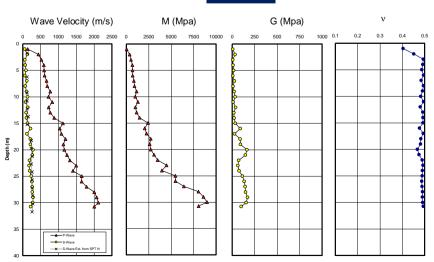
Downhole seismic test is an in-situ test and determine the velocity of primary (P) and secondary (S) seismic waves to provide the elastic soil parameters. The P and S waves velocities are used in geotechnical foundation analysis, static and dynamic soil analysis, liquefaction assessment and etc.
