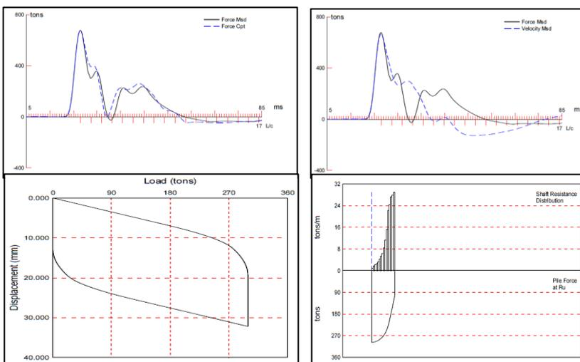
Pile Dynamic Analyzer (PDA), also called high strain dynamic load test, is based on monitoring the response of a pile subjected to hammer blows applied at the pile head. This method is widely used to estimate the bearing capacity and the integrity of the pile, as well as hammer performance, pile stresses, and soil dynamics characteristics, such as soil damping coefficients and quake values. This test is easy, fast, inexpensive and required small working area.
