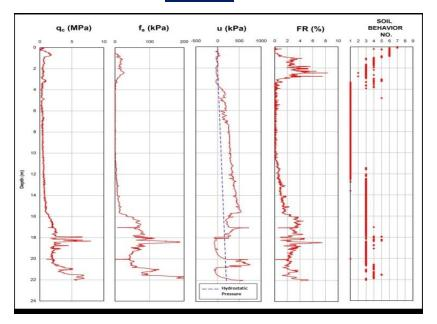
The Cone Penetration Test (CPT) is an insitu test developed in early 1920s. This test is mainly used for sites where there are deep deposits of transported soil such as in flood plains, river deltas, and along coastlines. The CPT test is fast to perform, economical, and it provides continuous record of cone resistance, sleeve friction and pore water pressure against depth.
