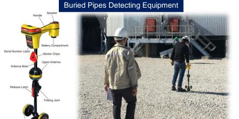
uses electromagnetic signals to determine the depth, direction and orientation of conductive underground cables and pipes. It consists of signal generator to apply signal to buried line then a handheld receiver locates the signals from the transmitters or naturally occurring passive signals from buried lines.
