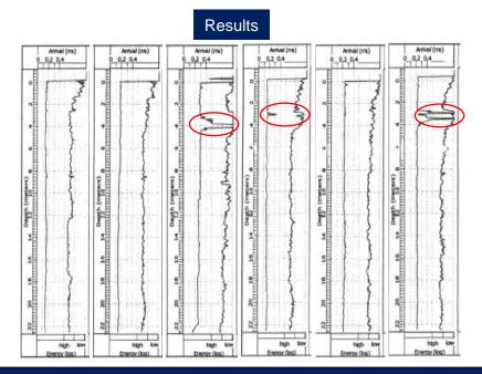
Crosshole sonic logging test is mainly used to check the integrity and homogeneity of the concrete in deep foundations and is also used for diaphragm wall, barrettes and dams. This test provides the propagation time and the relative energy of an ultrasonic pulse between parallel access installed in the pile or structure which is used to determine the quality of concrete and the poor zone of concrete.
