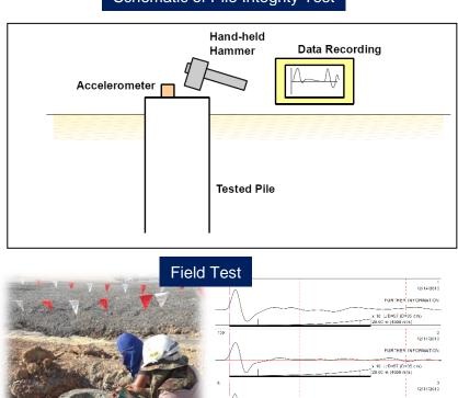
Schematic of Pile Integrity Test
