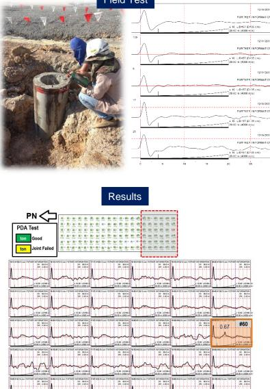
Low strain integrity test, also known as pile integrity test, is a non-destructive insitu testing to evaluate the pile integrity, pile dimensions, continuity and the consistency of the pile material. This test is quick and cheap to conduct method.
