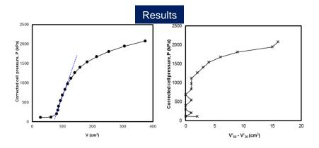
Pressuremeter test is an in-situ test that is performed to obtain the in-situ stress-strain behaviour of the soil. This test provides deformation modulus, undrained shear strength for clays or weak rocks, angle of shearing resistance for sands, angle of dilation for sands and in-situ total horizontal stress.
