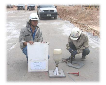
The field density test is a field control test for the compaction soil or any other pavement layer. The Field Density test by the Sand Cone Method was carried out in accordance with ASTM D1556-00 "Standard Test Method for Density and Unit Weight of Soil in Place by the Sand-Cone Method.
